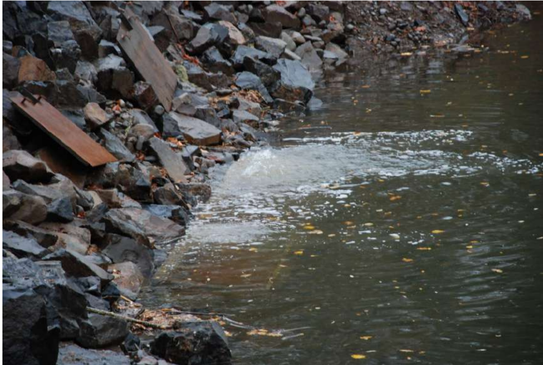
Photograph 19: View east at intake structure during test of fish screen cleaning jets (11/11/08).
